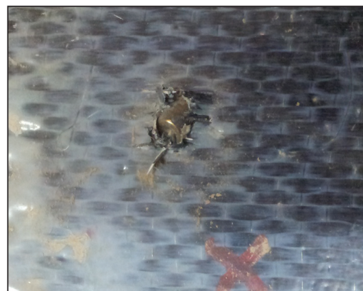
Fig. (4): The front face of hybrid plate (5)mm thick [6 layers E-Glass and 6 layers Carbon fibers]
