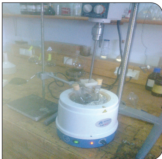
Fig. (1): Setup of Manufacture foam material of PVA
