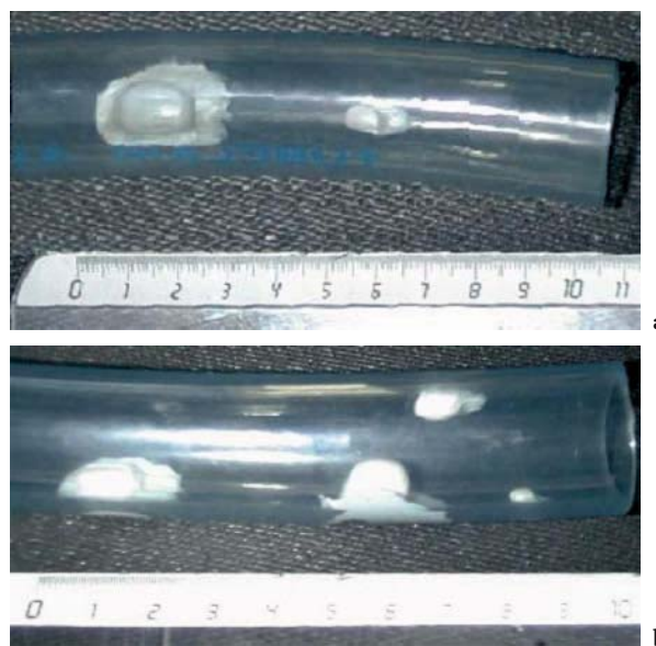
Fig. 18.5a,b. Parts of the tube phantom with inbedded plasticine beads
