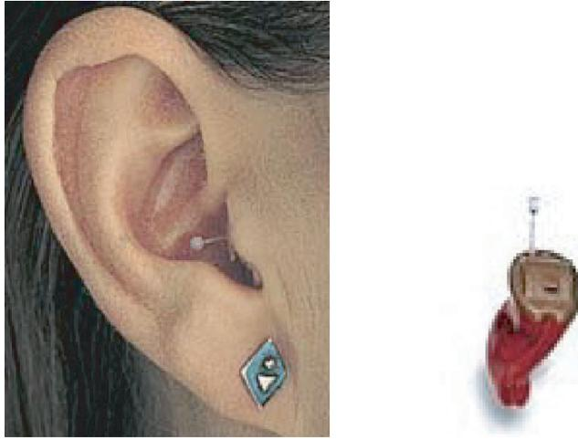
**FIGURE 22:** CIC style with a protruding cord to remove the device.
