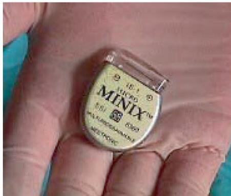
**FIGURE 32:** Typical pacemaker pulse generator with epoxy top for connection to leads.
