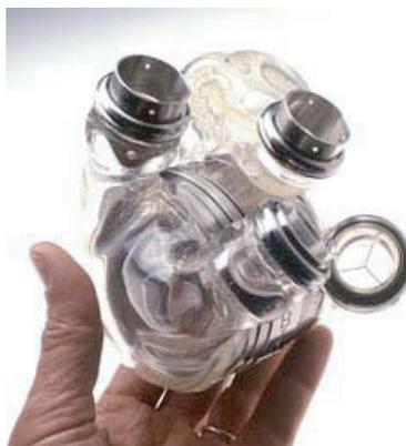
**FIGURE 15:** Biventricular electrically operated pusher plate design for a blood pump with four valves similar to that of the natural heart.
