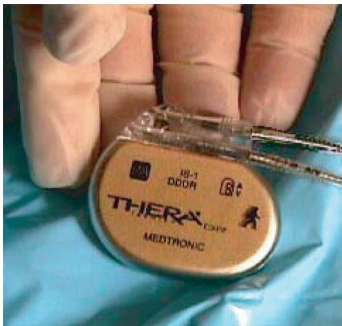
**FIGURE 33:** Pulse generator with leads attached.
