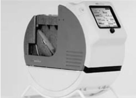
**Figure 15.2** Lifebridge B2T is one of the first fully portable emergency life support systems for patients suffering cardiogenic shock. First introduced in 2005, currently it has a CE mark for use all over Europe. It measures 61 × 45 × 37 cm and weighs 17.5 kg with an ability to generate up to 6l/minute flow with peripheral or central arterio-venous cannulation.
