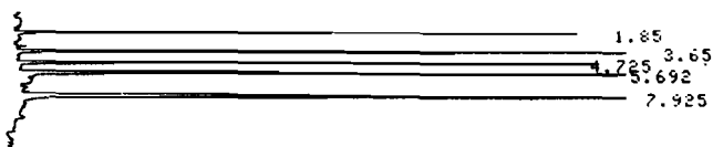
Figure 25-2. Separation of four aromatics with a 2 mm micro-bore column using a flow of 220 \mu l/min.
