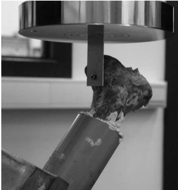
Fig. 22. Set-up for testing the strength of the screw-bone fixation: a screw is fixed in the cadaver bone and transversely loaded.
