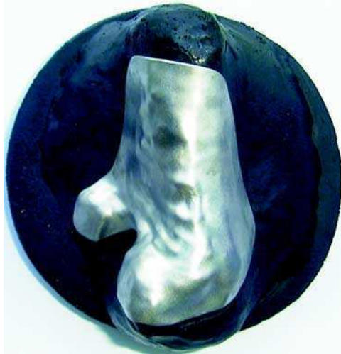
Fig. 16. Titanium membrane on mould.
