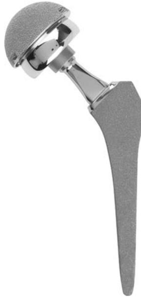
**Figure 6.5** A typical total hip joint replacement is made primarily of metal. The ball of the femoral hip stem fits into a pelvic acetabular cup that is lined with ultra high molecular weight polyethylene (UHMWPE) for friction-free motion. (Photograph of the PROFEMUR<sup>®</sup> Z minimally invasive hip stem with modular necks courtesy of Wright Medical Technology, Inc.)
