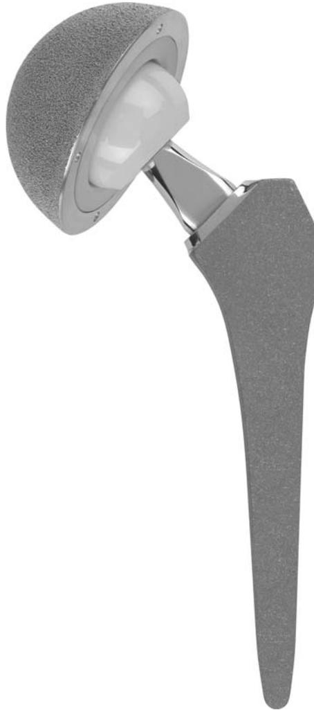
**Figure 6.10** In this artificial hip joint, the polymer bearing surface and some of the metallic components have been replaced by ceramics to improve the durability of the joint replacement. This design features a ceramic femoral head and acetabular cup. (Photograph of the LINEAGE<sup>®</sup> ceramic-ceramic acetabular cup system is courtesy of Wright Medical Technology, Inc.)
