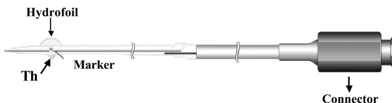
FIGURE 9.1 Coronary thermography catheter. A thermistor (Th) is positioned at the distal part. Opposite the thermistor is a hydrofoil that facilitates the contact of the thermistor with the vessel wall. At the proximal part, the connector for the thermistor lead wires is demonstrated.
