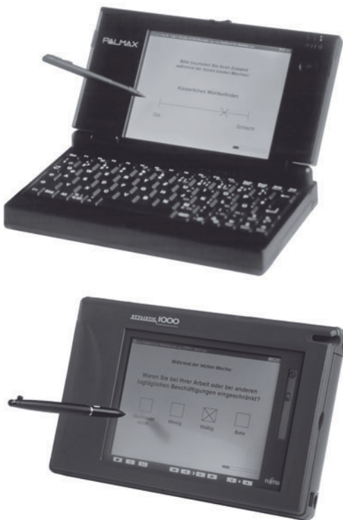
Fig. 7.1 Implementation of the QoL-Recorder on a Palmax PD-1000 Mini-Pen Computer and a Fujitsu Stylistic 1200 Pen Computer.
