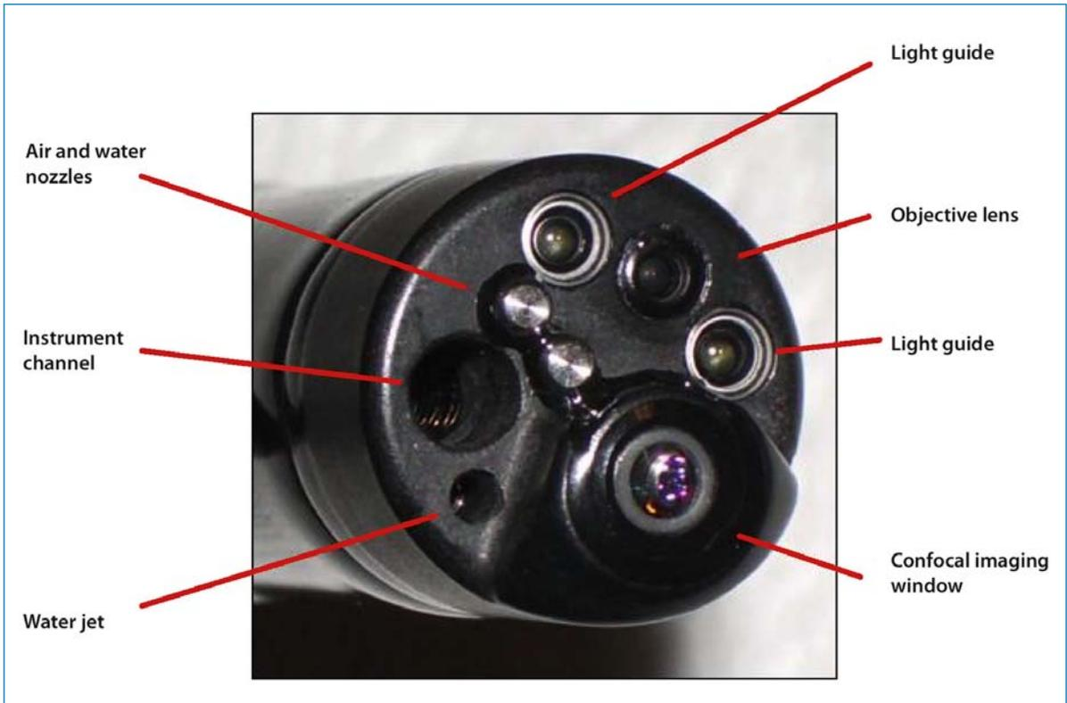
**Fig. 4.2.** The distal tip of the confocal endoscope contains the scan mechanism and the confocal imaging window. The instrument channel measures 2.8 mm, the outer diameter of the endoscope is 13.2 mm. The endomicroscope contains two light guides
