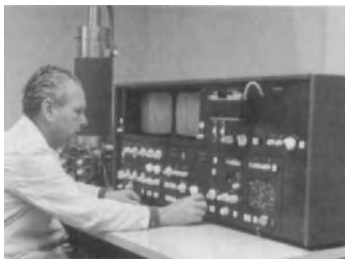
FIGURE 69. The first Czechoslovak scanning microscope: the Tesla BS 300, operating between 1 and 50 kV, and with secondary, back-scattered, and absorbed current imaging modes, slow scan and TV-rate imaging, and twin-screen display.
