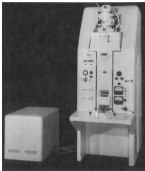
FIGURE 8. CSF Electrostatic electron microscope type M III. A very early postwar series production instrument. Accelerating voltage 50 kV, with a telefocus gun.
