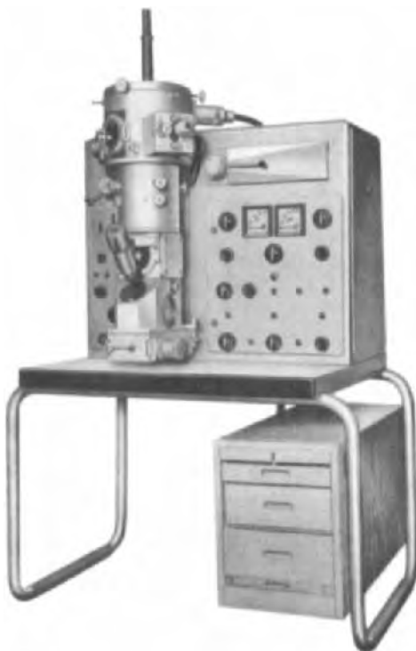
FIGURE 55. Model EF 6 on EF 4 base, made by Zeiss Jena. This emission microscope could operate at temperatures up to 1000°C, and had facilities for secondary electron imaging from electron or ion beams.
