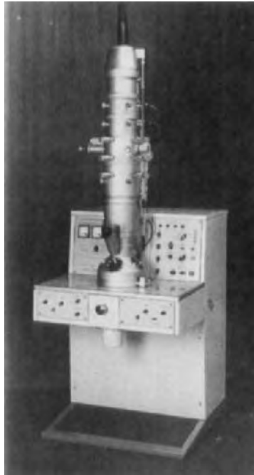
FIGURE 48. WF (TV factory) SEM 3-2. An advanced design of TEM with four imaging lenses and a built-in anticontaminator. Options for a heating stage and a high-resolution electron diffraction stage.
