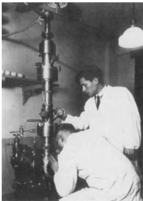
FIGURE 2. General view of the Mark I transmission electron microscope with two-stage magnetic lenses built in 1939. On the right is the young Prof. E. Sugata.
