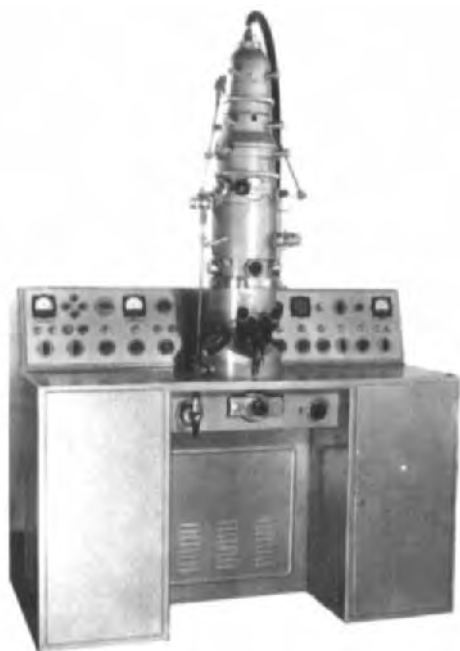
FIGURE 29. An early microscope from the USSR. The EM 5 instrument was manufactured both in Krasnogorsk and in Sumy. It had three imaging lenses but a single condenser. The objective was fitted with an octupole stigmator.
