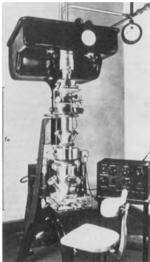
FIGURE 4. Siemens production prototype of the ÜM, showing “bathtub” around the electron gun. The imaging length is still 800 mm. Late 1938. (Reprinted with permission from Ruska, E. (1980).)
