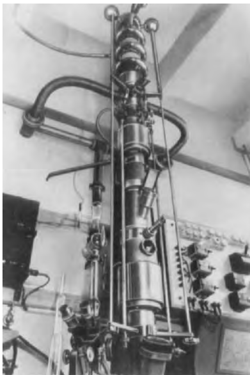
FIGURE 13. Wartime (1940–1944) development of a high-voltage TEM. Prototype for TEMs working above 200 kV.
