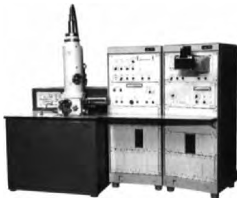
FIGURE 68. The Sumy REM 200 scanning microscope with voltage range 5–40 kV, and magnification range 40–80,000. The first SEM with large-scale production in the USSR.
