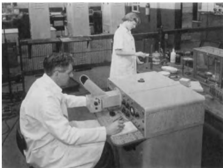
FIGURE 17. Metro-Vick electron microscope type EM 4. Simplified 50-kV console instrument, with double-projector lens and triple specimen holder. At the controls, M. Venner, author of the paper, "Where to Kick the Electron Microscope." Power supply cabinets of the EM 3 instruments appear in the background.
