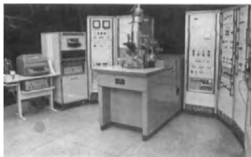
FIGURE 8. KYKY prototype ion-microprobe mass analyzer (1978): spatial resolution 2 m at 20 kV, mass resolution 2000, sensitivity, 2 parts per billion for boron in silicon.
