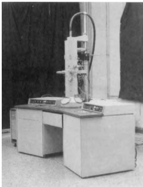
FIGURE 9. KYKY DX-4 (1980), resolution 0.2 nm, 100 kV: the first microprocessor-controlled TEM in China.
