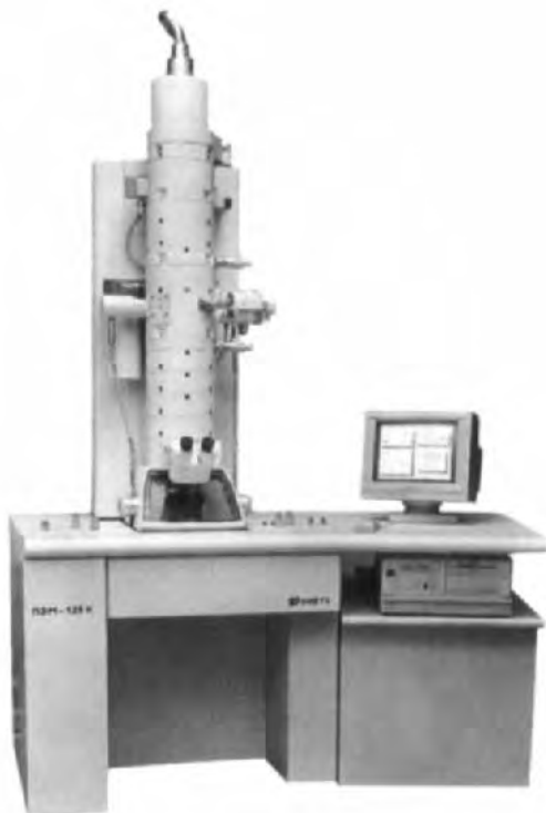
FIGURE 82. Sumy PEM 125K, a computer-controlled high-resolution microscope for materials science. Resolution 0.35 nm at 60° tilt.
