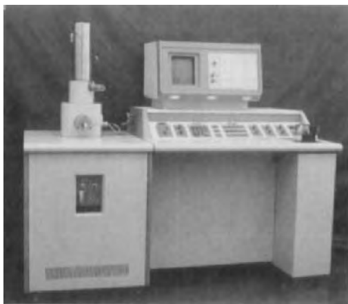
FIGURE 21. DXS-10A (1992): resolution 10 nm, 30 kV; some automatic features (Shanghai Factory).
