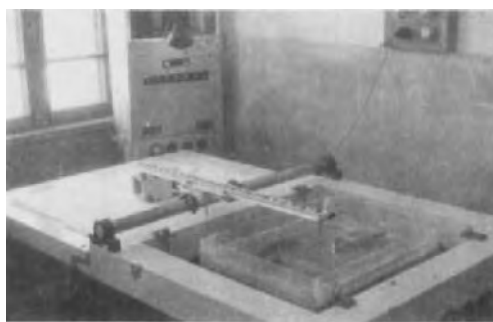
FIGURE 5. KYKY electrolytic tank and trajectory tracer, with space-charge simulating electrolytic tank (1963). The current-injecting needles are at the bottom of the tank.
