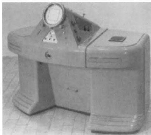
FIGURE 11. Philips EM 100. First 100-kV electron microscope with four imaging lenses, selected-area diffraction facilities, and a focus wobbler, 35-mm camera.
