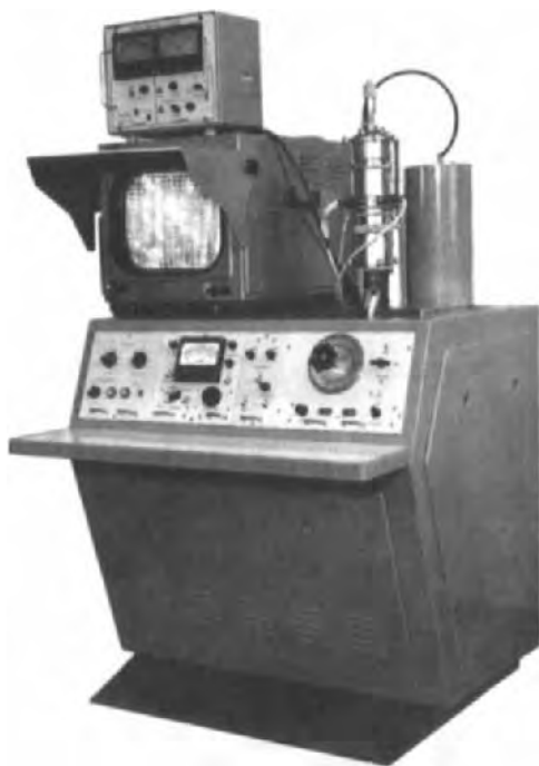
FIGURE 40. Scanning microscope REMN-1 from Sumy. The first scanning microscope manufactured in the USSR. Operated at the very low voltages of 0.5–2.3 kV, it had only absorbed current detection.
