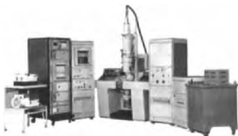
FIGURE 66. Electron diffraction camera EMR 100. Besides the physically determined camera lengths, a lens between the specimen and screen allowed for much longer effective camera lengths for the examination of large diffraction spacings.
