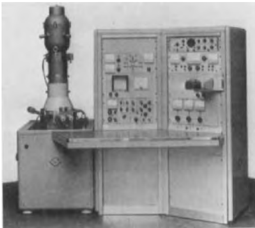
FIGURE 39. Cambridge Instruments Stereoscan 1. The first commercial scanning microscope in series production: 20 kV, resolution 50 nm.
