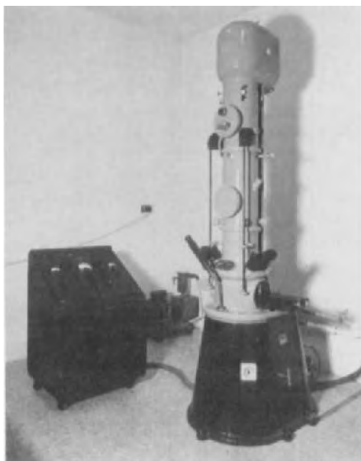
FIGURE 10. Metro-Vick EM 2. Note the very long column enclosing the lenses, and the separate console with lens supplies. The monocular viewer was a nonstandard addition.
