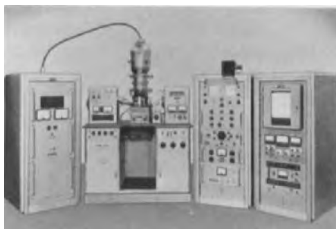
FIGURE 36. Cambridge Instruments Microscan 1. The first scanning electron probe micro-analyzer. Two semifocusing X-ray spectrometers. Note the bulky electronics required at that date.
