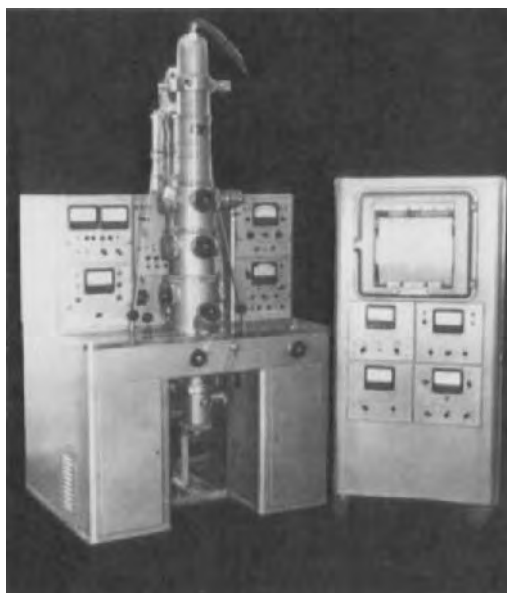
FIGURE 56. Electron diffraction camera type EVR-1, manufactured in Sumy. Operated at 40–60 kV. Ports for three camera lengths.
