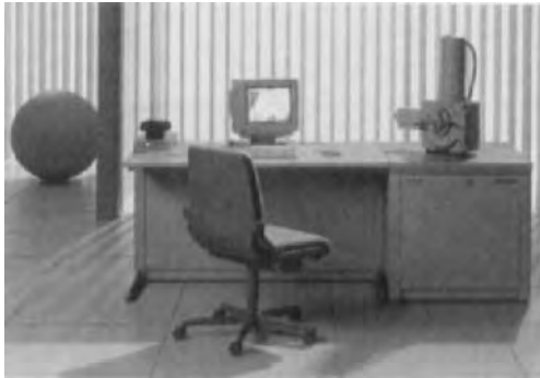
FIGURE 77. Philips XL 20 desktop scanning microscope. The logical conclusion of computer control—all normal control knobs are replaced by a mouse-operated menu system.
