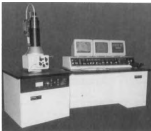
FIGURE 11. KYKY 2000 (1989): digital SEM with 512 \times 512 frame grabber and image processing software.
