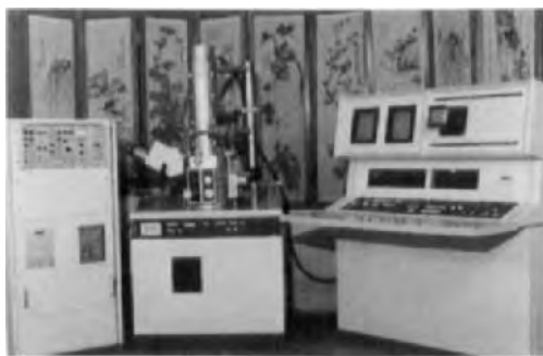
FIGURE 14. DXS-3 SEM (1989): resolution 6 nm, 35 kV, with mini wavelength-dispersive spectrometer (WDS) (Nanjing Factory).
