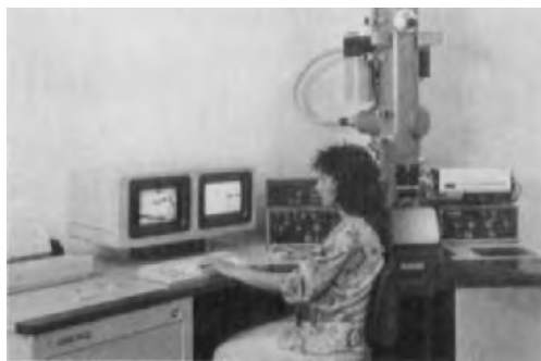
FIGURE 80. Zeiss CEM 902. Computer-controlled version of EM 902, the analytical microscope with energy-loss imaging and energy spectroscopic imaging.
