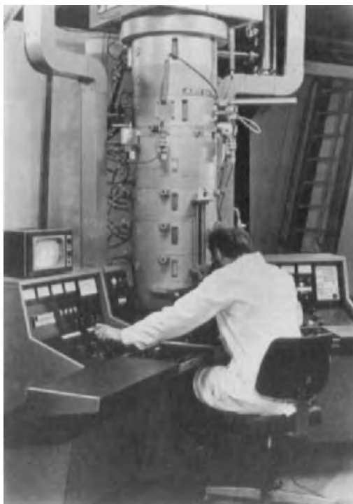
FIGURE 59. AEI EM 7. 1000-kV high-voltage electron microscope. First with nonrotational image with change of magnification. Many special in situ treatment stages.
