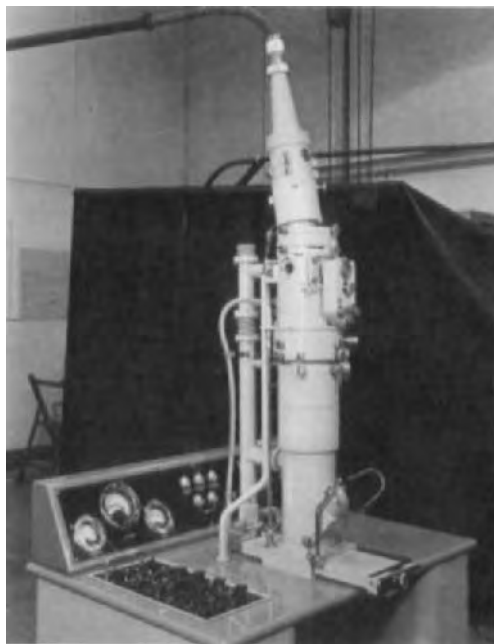
FIGURE 26. Metro-Vick electron microscope type EM 3A, showing the gun and condenser tilted at 8^\circ for reflection microscopy, and the reflection stage in position above the objective.
