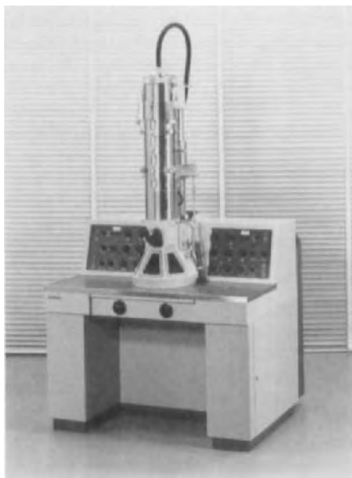
FIGURE 31. Philips EM 200. Solid column construction with lens alignment carried out by movements of polepieces.
