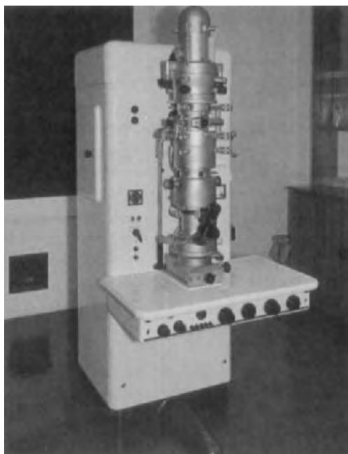
FIGURE 30. Siemens electron microscope type Elmiskop I. The first high-resolution electron microscope (1 nm). Perhaps the most important single development in the history of commercial instruments. The first instrument with a double condenser and two stigmators.
