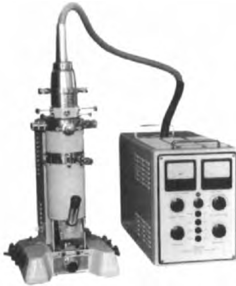
FIGURE 28. Tesla type BS242. First (and only) European tabletop microscope, 60 kV, four lenses. It was in widespread use, particularly in Eastern Europe.
