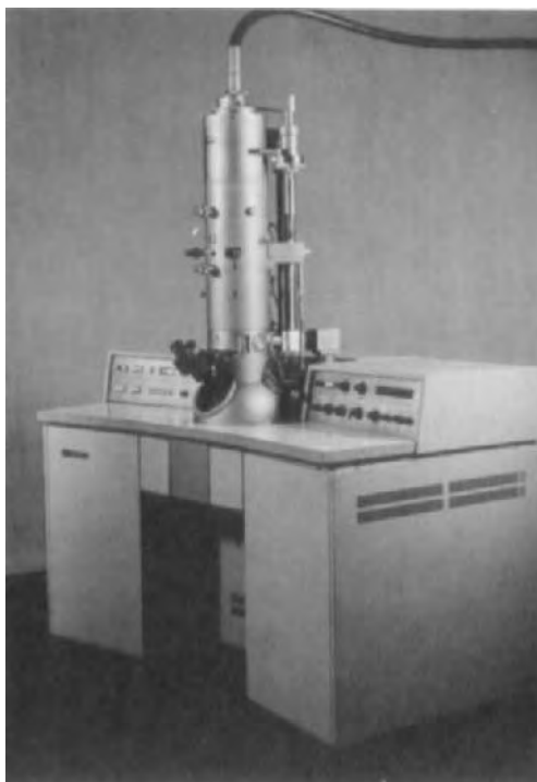
FIGURE 17. DXT-10 TEM (1976): resolution 1 nm, 100 kV (Nanjing Factory).
