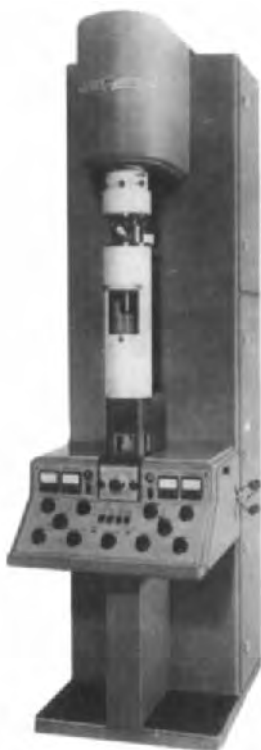
FIGURE 25. Tesla electron microscope type BS 241. The first Czech microscope, showing its evolution from the RCA EMU 2A.
