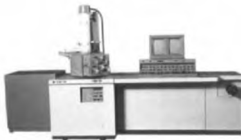
FIGURE 75. Sumy REM 101 SEM, 0.2–40 kV, 5 nm. A range of instruments for different applications, and when fitted with two fully focusing spectrometers, known as the REMMA 202M.
