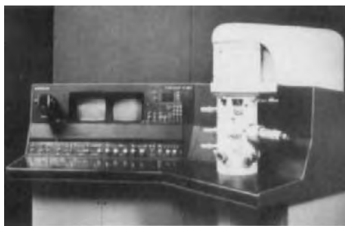
FIGURE 73. Siemens ST 100F. The first European field-emission STEM; with bright- and dark-field secondary electron detectors. X-ray analyzer, and electron energy-loss analyzer with magnetic-sector spectrometer.
