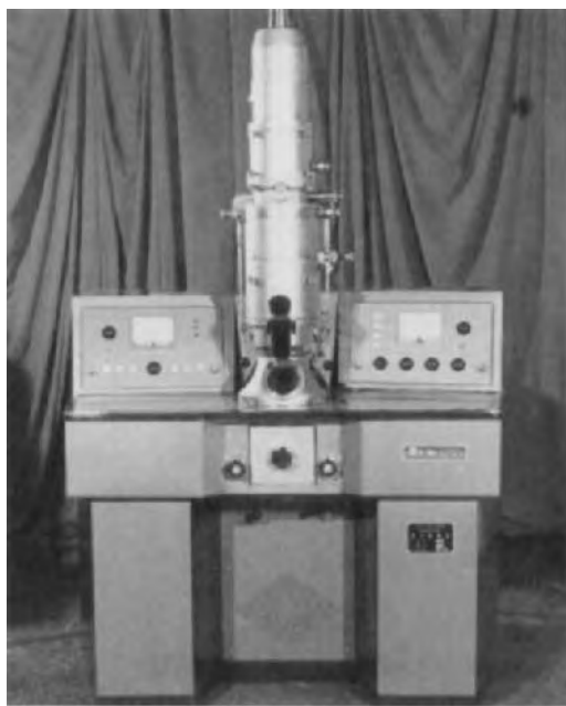
FIGURE 16. XD-201 TEM (1967): resolution 2 nm, 80 kV (Nanjing Factory).
