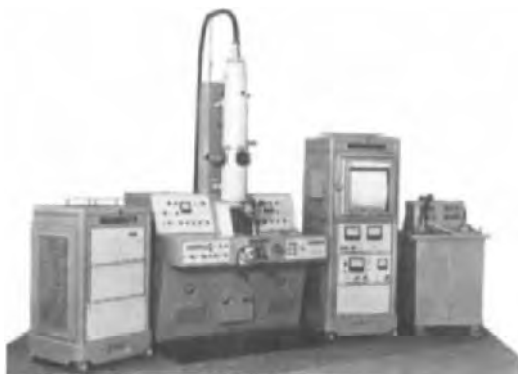
FIGURE 57. Diffraction camera ER 100, introduced in 1967. Voltage range 25–100 kV.
