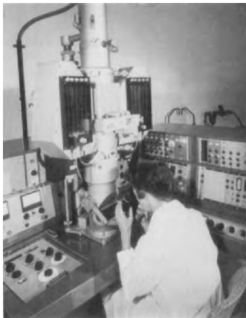
FIGURE 58. AEI EMMA-4 electron microscope-microanalyzer. The first analytical TEM designed as an integrated instrument. Two fully focusing spectrometers. Spot size reduced to 0.13\text{ }\mu\text{m} by use of a minilens as condenser 3.
