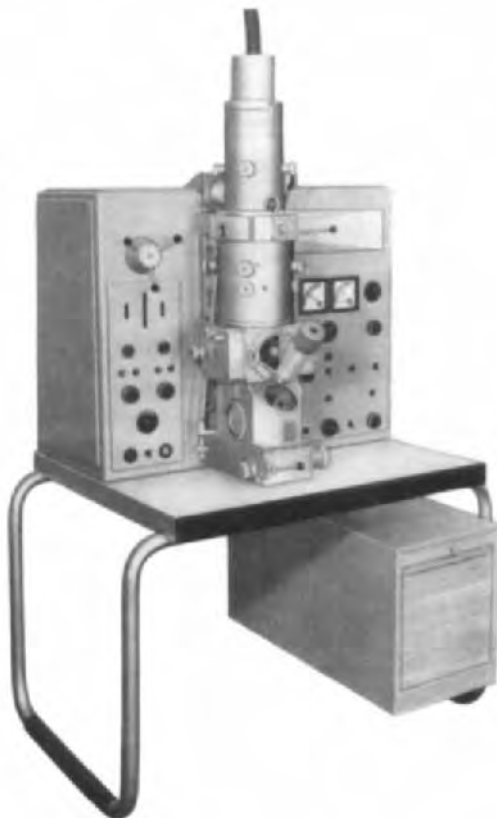
FIGURE 45. Carl Zeiss Jena model EF 4 modular microscope for transmission and reflexion microscopy and diffraction.
