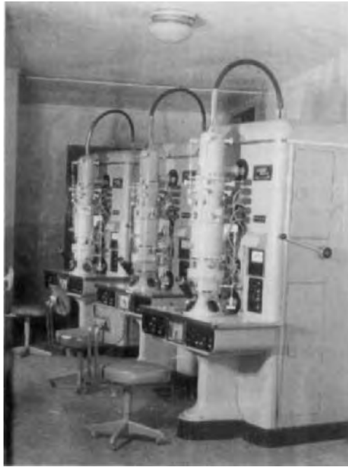
FIGURE 18. Three DXA4-10 TEMs on test (1968): resolution 0.7 nm, 100 kV (Shanghai Factory).
