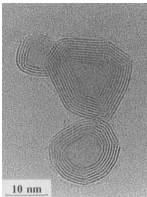
FIGURE 1. High-resolution TEM image of a new form of tungsten disulfide ( \text{WS}_2 ) taken by the author in a 400-kV TEM (point resolution 0.16 nm). This compound normally occurs in the form of sheets, but here they have curled up to form closed shells. The dark contrast in the concentric shells corresponds to layers of tungsten atoms, seen edge-on. Variations in the relative stacking of successive tungsten layers can also be discerned in such images. This new structure is an unexpected analog of the well-known "buckyballs" and "bucky-onions."
