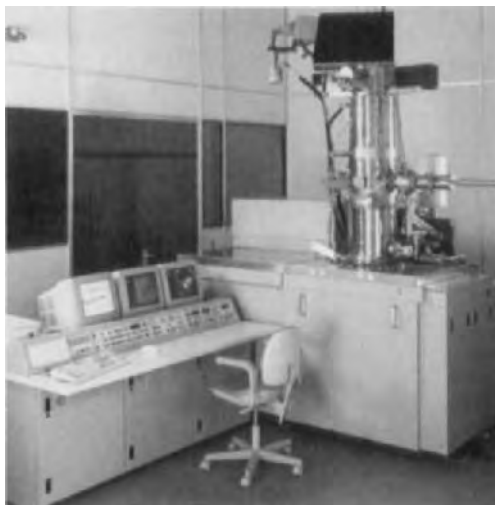
FIGURE 83. Vacuum Generators HB 603. The first field-emission STEM instrument operating at 300 kV. Ultrahigh resolution; with wide-angle detector for incoherent imaging giving atomic number contrast.
