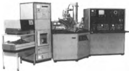
FIGURE 74. Sumy REM 100U. Universal scanning microscope with heating and straining stage, STEM operation, and facilities for characterizing dielectric specimens. Eucentric stage.
