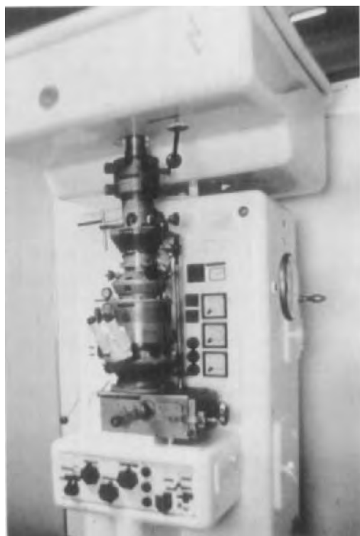
FIGURE 5. Siemens ÜM electron microscope, the world's first series production instrument. First production of polepiece lenses. Initially worked up to 70 kV, resolution 7 nm. Equipped with desk, short-focal-length objective, specimen and camera airlocks, and viewing telescope.
