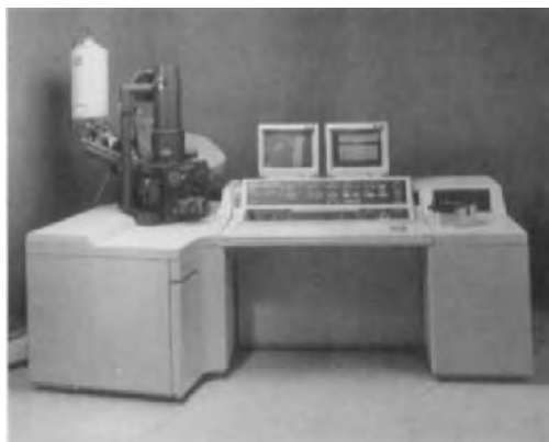
FIGURE 76. Cambridge Stereoscan S.360 with computer control, image store, and central image processing. The column is fitted with an X-ray solid-state detector and a focusing spectrometer.
