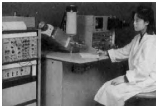
FIGURE 13. Mini-SEM DXS-X2 (1983): 15 nm, 25 kV (Nanjing Factory).
