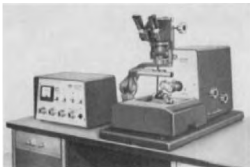
FIGURE 12. The well-known Ultratome microtome manufactured by the LKB Company. More than 4000 units were manufactured.
