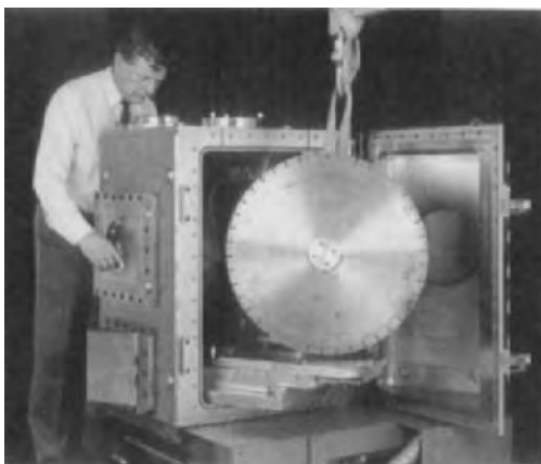
FIGURE 70. Camscan Series 3 with designer Dick Paden, with a special large specimen chamber for bulky specimens. Pioneer of modular construction offering special facilities.
