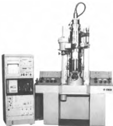
FIGURE 65. Electron microscope/microanalyzer EMMA 4, based on the EMV-100B. This was the last dedicated EMMA to be produced in Europe.
