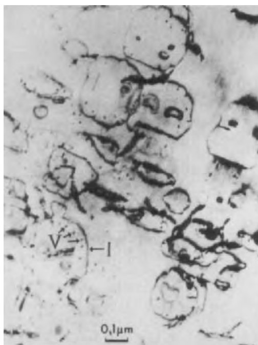
FIGURE 8. Complex dislocation loops introduced in thin KBr by two-step electron irradiations: I, interstitial type; V, vacancy type (Kawamata, 1976).
