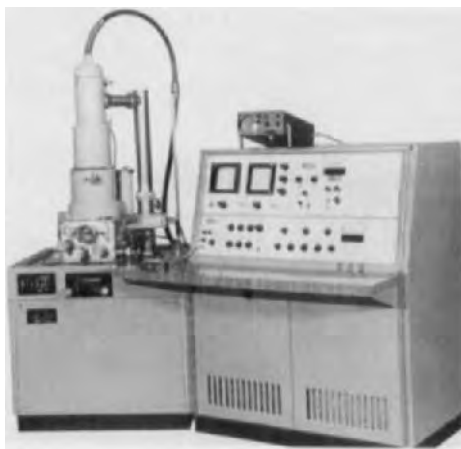
FIGURE 7. KYKY DX-3, resolution 10 nm, 30 kV (1975). The first Chinese scanning electron microscope.
