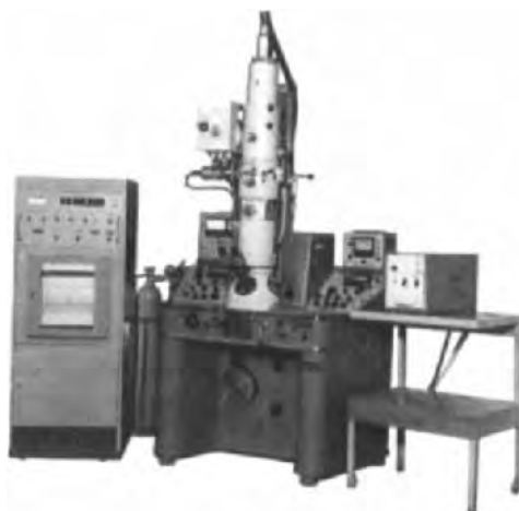
FIGURE 64. Electron microscope/microanalyzer EMMA 2, based on the Sumy TEM UEMV-100.
