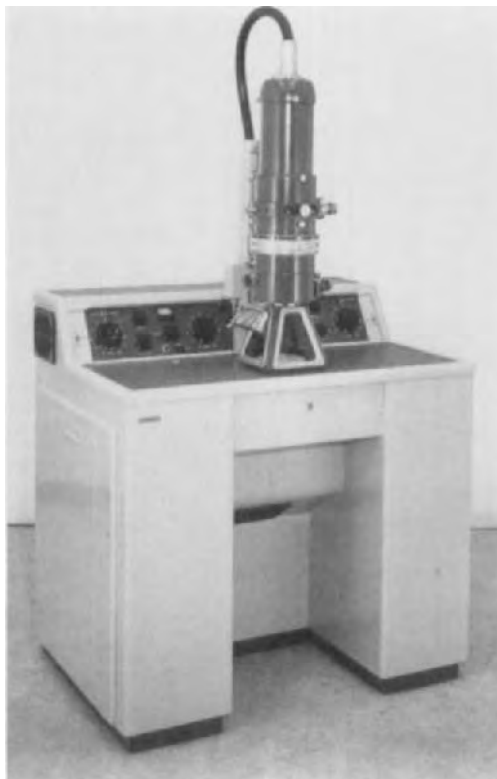
FIGURE 20. Philips electron microscope type EM 75. Simplified 75-kV instrument with very-short-focal-length objective and a fixed excitation projector lens unit with a subsidiary variable polepiece gap. Objective lens supplied by a power pack with selenium rectifiers and smoothing condensers.
