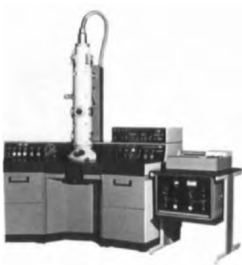
FIGURE 84. Electron diffraction camera EMR 102 with digital recording of information. A later modification included automatic measurement of the information and computer processing of diffraction patterns.
