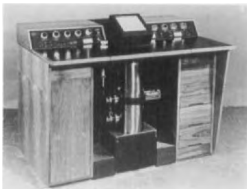
FIGURE 63. AEI Corinth 275. A console-type microscope with inverted column for routine applications. It had a four-specimen holder in a simple airlock, and large screen viewing.
