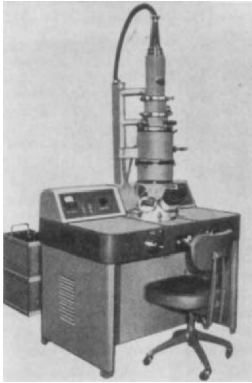
FIGURE 5. Model HS-6 electron microscope, provided with a permanent magnet lens system (1958).
