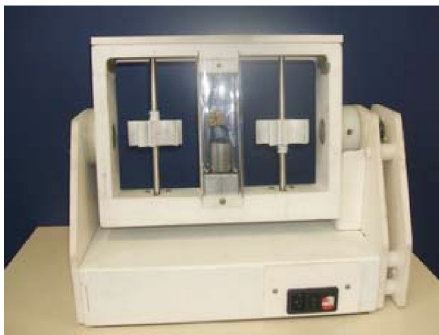
FIGURE 3.20: Microgravity Centre 3D clinostat ( http://www.pucrs.br/feng/microg ).
