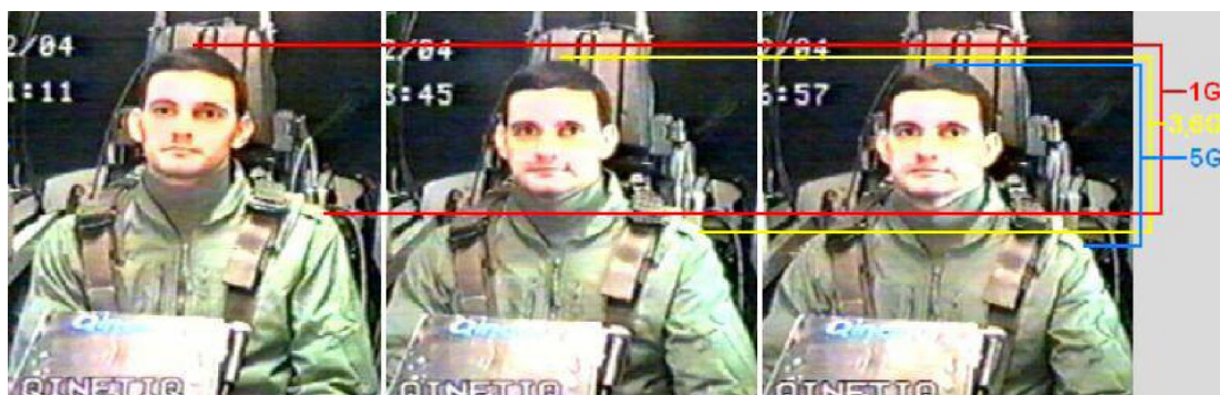
FIGURE 2.14: Test subject during hypergravity exposure at the Royal Air Force human centrifuge in Farnborough, England. Note the progressive decrease in height from +1G to +5Gz ( http://www.pucrs.br/feng/microg ).
