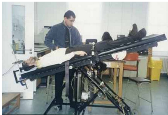
FIGURE 3.1: Subject during an HDT experiment—KCL tilt table ( http://www.pucrs.br/feng/microg ).
