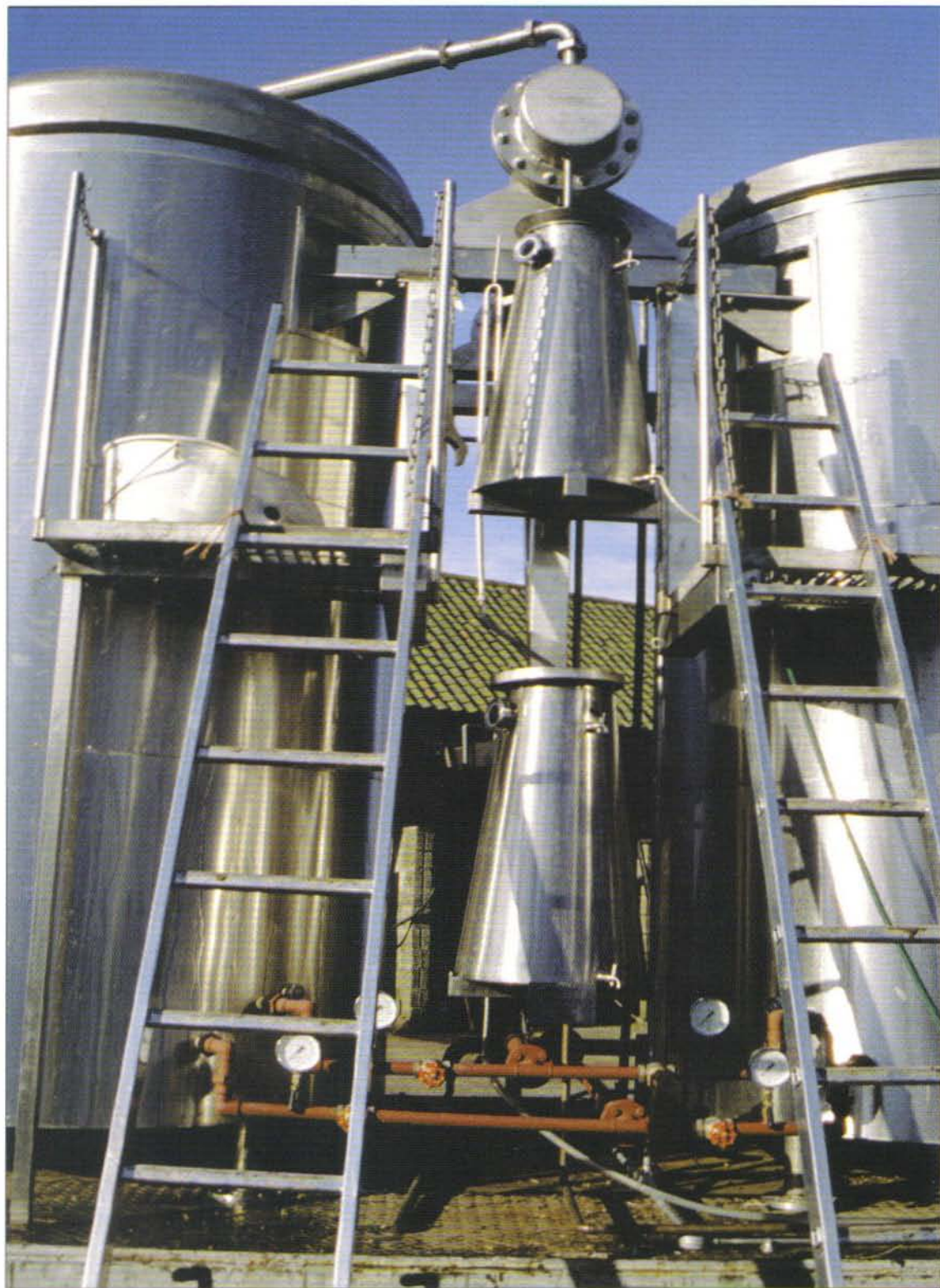
Mobile distillation unit being used for chamomile oil extraction (Norfolk, Anglian Essential Oils Ltd.)
