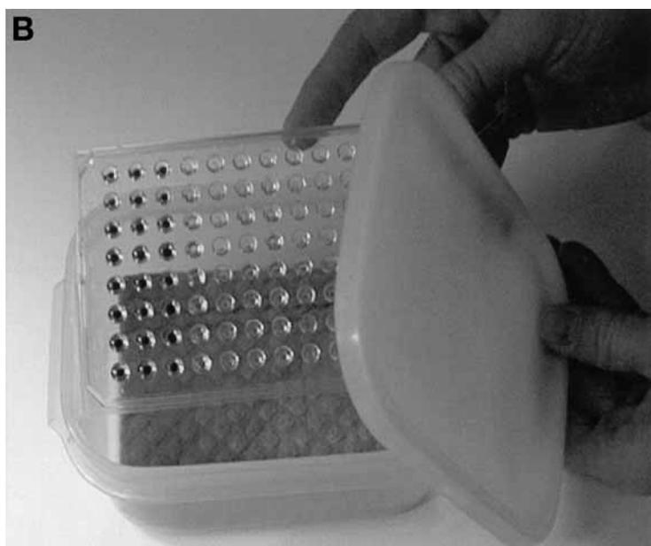
**Fig. 3.** Microbatch in 96-well plates. **(A)** Transfer of oil from the reagent basin to the Imp@ct™ microbatch plate with a multichannel pipet. The first three rows at the bottom of the photograph show coalesced droplets of the protein and screening solutions under the oil. **(B)** Storage of the plate in a plastic sandwich box with a wetted sponge towel.
