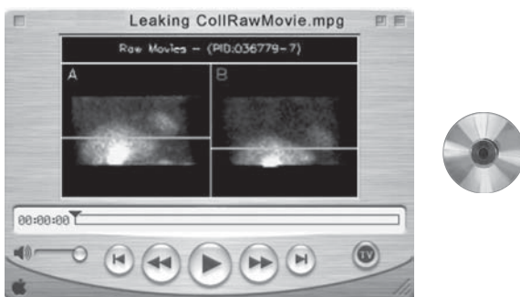
Fig. 14-52. Rotating stress (A) and rest (B) planar projection images. During the rotation of the stress images a bright “glow” appears on the top of the images in the anterior positions. This is most likely due to “leaking” radioactivity from outside the field of view between the mounted collimator and the gamma camera detector head. The technologist must investigate the cause of this artifact by surveying the patient’s gown, neck, and arms for contamination or extravasation of injected dose. It is also possible that the collimator is not mounted correctly on the camera head. This is potentially dangerous because the collimator could fall off and injure the patient. If the collimator is mounted correctly, one can purchase lead guards that cover the slit between the collimator and camera and will prevent this artifact from recurring.
