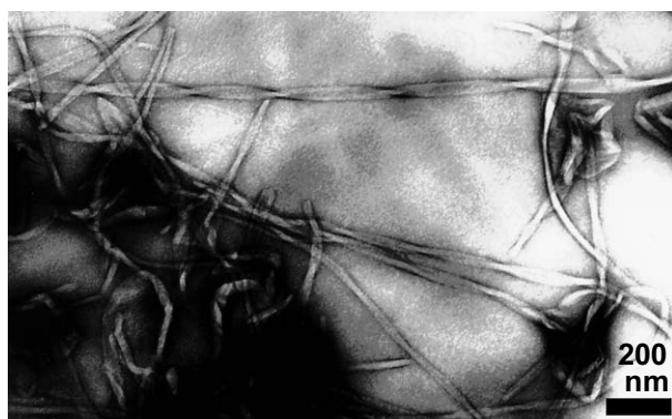
FIGURE 18.3 Transmission electron micrograph of helical superstructures self-assembled from 10 and 11 in water. 34
