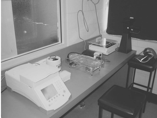
Figure 13.3. A simple laboratory PCR setup based around the BioRad iCycler system.
