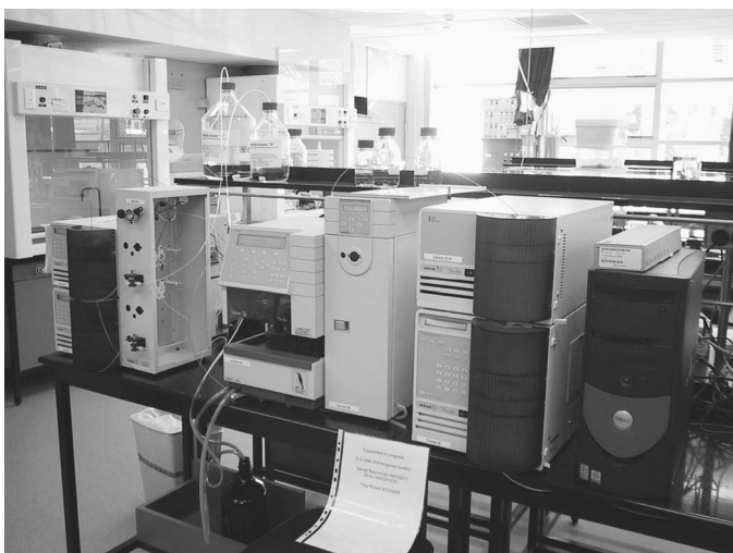
Figure 13.1. A dHPLC designed for the detection of new and potentially interesting SNPs in candidate genes.
