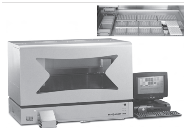
Figure 3.6 The Qiagen BioRobot M48. The workstation is equipped with special anti-contamination features, such as a completely enclosed robotic deck. Reproduced with permission from QIAGEN Products
