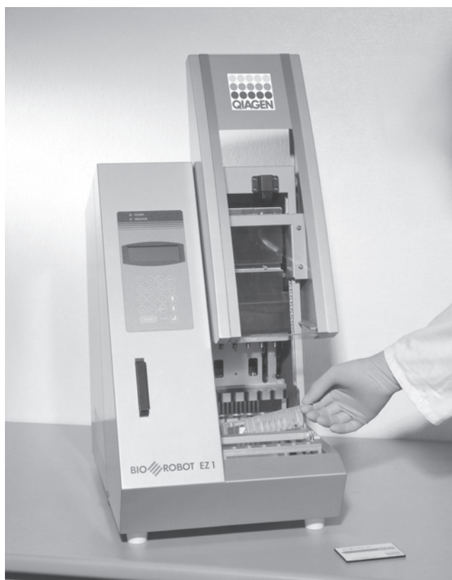
Figure 3.5 The Qiagen BioRobot EZ1. The EZ1 working deck has six slots to take the kit cartridges, an aligned tube rack to locate tubes for samples and re-suspended DNA and, above the deck, a robotic head with six positions, each having a spike for piercing the foil seals on the cartridges, a pipette and a magnetic probe. Reproduced with permission from QIAGEN Products
