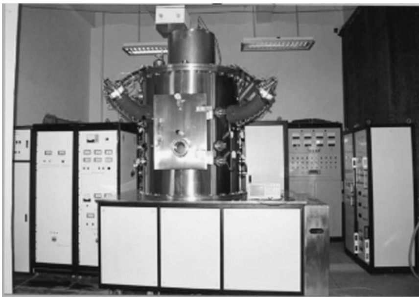
FIGURE 19.8 Photograph of the third-generation plasma immersion ion implanter. (From Chu, P.K., Rev. Sci. Instrum. , 72, 1660, 2001. With permission.)
