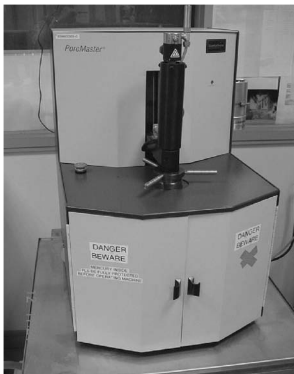
FIGURE 5.10 Mercury porosimeter instrument for the measurement of scaffold porosity.
