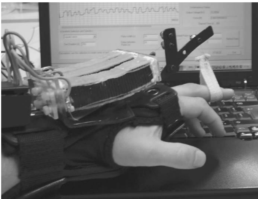
FIGURE 16.13 Prototype sample of a dynamic hand splint equipped with dielectric elastomer actuators.
