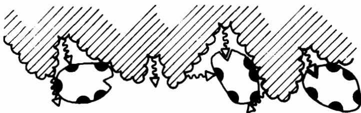
Fig. 4.18. Schematic illustration of the effect of concentration of an immobilized affinity ligand and uneven surface of a solid carrier on specific and nonspecific sorption.
