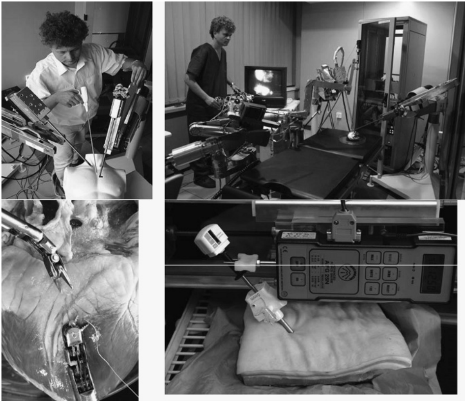
Figure 10(b) Comparison of different tools: Robin Heart 0,1 and laparoscopic tools; test of Robin Expert advisory system (presented by the author); and the test using animal tissue.
