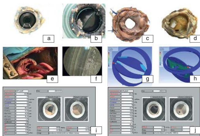
Plate 4 The samples of explanted valves collected in the Institute of Heart Prostheses, FCSD (COST Action 537 project). One-disk (a) and two-disk mechanical valve (b) and two bioprotheses (c,d). The in vivo valve test on ship (e). The microscopic evaluation of valve's disk (f) and modeling of mechanical valves – equivalent elastic strain values (g,h). The effect of biological heart valve prosthesis damage on hemodynamic efficiency has been investigated and analyzed: improper functioning due to leaflet calcification – the opening area of “calcified” (leaflets partially glued (i)) valve decreased by 44%, while the pressure gradient grew up to 22 mmHg. Perforation of a leaflet (j) – significant perforation (hole area 6.68 mm 2 ) of leaflet caused increase in back-leakage of 147% to 8.38 (6.8 ml). (See Figure 7 of chapter 1, p. 31).
