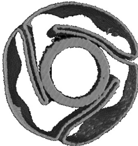
Figure 3 CT-Image reconstruction of tri-folded angioplasty balloon.
