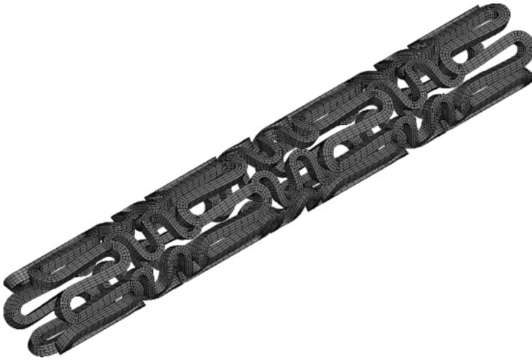
Figure 1 Approximate CAD model of Cypher stent and finite element discretization.
