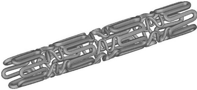
Figure 2 CT-Image reconstruction of Cypher stent.
