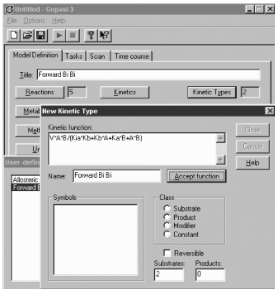
Figure 8.5. Definition of kinetic type for Gepasi. To define new kinetic type, open User-defined kinetic types dialog box by clicking Kinetic types button (Model definition page). Click Add button to open New kinetic type dialog box. Enter kinetic equation as shown in the Kinetic function box (forward ordered Bi Bi) of the inset and click Accept function button.
