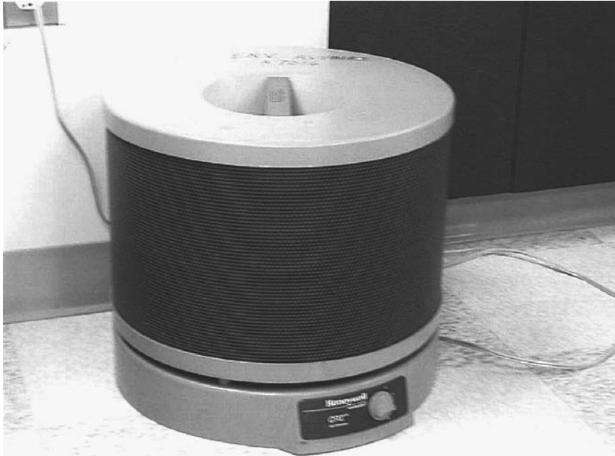
FIGURE 62.6 An in-room air-cleaning device that can be used to filter particulate and/or vapors within a room.
