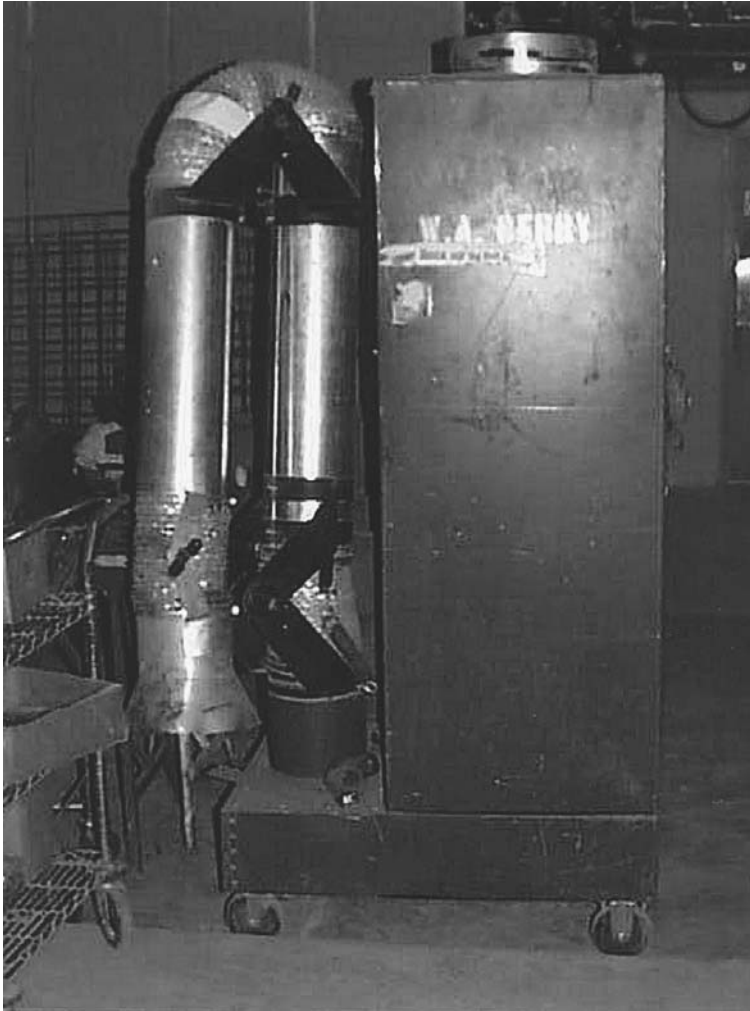
FIGURE 62.9 Welding fume extraction device used to capture and filter wet or dry fumes at their source.
