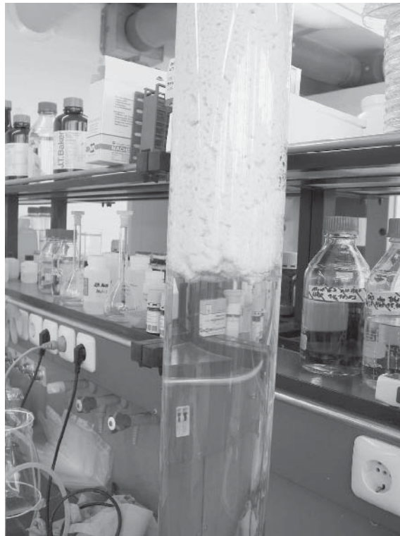
Figure 3.2 Bacterial alkaline lysate during (above) and after (below) flotation.
