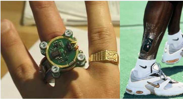
Figure 1.8 (Left) the first prototype ring sensor with RF transmitter powered by a coin-sized battery ( courtesy of Professor Harry Asada, MIT ). (Right) a FitSense sensor attached to an athlete's shin enabling measurement of stride length, step rate, instantaneous speed, distance, and acceleration ( courtesy of Tom Blackadar, FitSense Inc. ).
