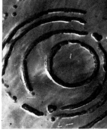
Figure 2. Micrographs of a replica from the 8 \cdot 10^{-4} mol/liter DDAB aqueous solution obtained by freeze-fracturing electron microscopy. 13 The distance between the layers is about 100 nm. The layer thickness and the size of individual vesicle (seen in the upper left corner of the micrograph) is about 20 nm.
